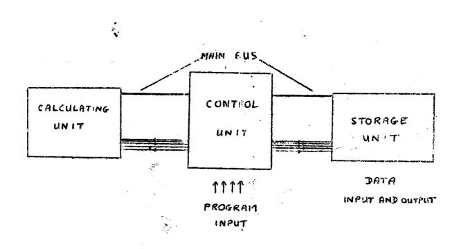
The K.G.S.1 digital computer performs simple calculations in binary arithmetic simulating the working of a full scale digital computer, although the actual calculations it can perform and the speed with which it performs them is strictly limited. In this computer a 1 digit is represented by a negative potential or a light on, and a 0 digit by zero potential or the light off.
